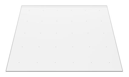
A simple phantom for quality assurance of geometric distortion and spatial resolution of gamma cameras. Array of holes, which when filled with activity, allows to measuring point-to-point distances and Point Spread Function (PSF) - spatial resolution - at each point and its homogeneity across the entire Field of View.
