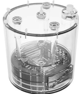
The phantom for **NM systems performance evaluation: routine quality assurance tests**, as well as extensive acceptance tests. It can be used to evaluate: pixel size, spatial linearity, RMS noise, signal to noise ratio (SNR), slice width, uniformity, spatial resolution, point spread function, slice position verification, slice incrementation, accuracy, center of rotation, verification, volume sensitivity and low contrast sensitivity.
