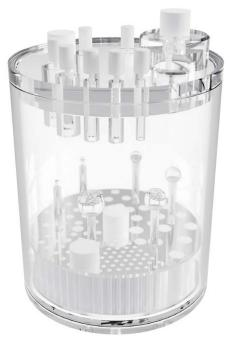
The phantom for small FOV NM and PET systems performance evaluation (collimator, artifacts, calibration, reconstruction parameters) Among other things, it can be used to evaluate: center-of-rotation error, non-uniformity artifacts, changes of radius-of-rotation on spatial resolution, reconstruction filters on spatial resolution, attenuation and scatter compensation.
