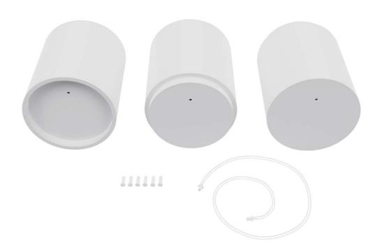
The PET scatter phantom is an acceptance testing tool used to determine the imaging systems relative sensitivity to scatter radiation. It can be used to measure the effects of dead-time and the effects of random events generated at different levels of activity of the line source.
