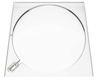
Flood phantoms provide a simple and efficient means of obtaining optimum camera performance with respect to uniformity of response over the entire crystal area. These phantoms are designed to be filled in horizontal position, thus preventing slight bulging caused by water pressure during vertical filling. Therefore, better uniformity in distribution of activity can be achieved.
