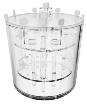
This module can be used as a standalone in air or in water if mounted in the Pro-NM Performance cylinder. It can be used to evaluate changes of radius-of rotation on spatial resolution, spatial resolution measurement in air and in water, quantitative evaluation of reconstruction filters and scatter compensation methods.
