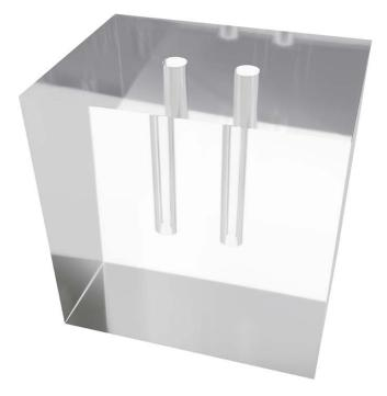
This scatter phantom simulates in-vivo forward and backscatter characteristics of 99mTc gamma rays for the extrinsic measurement of a scintillation camera's deadtime. The phantom produces a spectrum typical of that observed from 99mTc in the myocardium. Reference: Ralph Adams, Gerald J. Hine, and C. Duane Zimmerman, "Deadtime Measurements in Scintillation Cameras Under Scatter Conditions Simulating Quantitative Nuclear Cardiography," The Journal of Nuclear Medicine, 19 (1978), 538-544.
