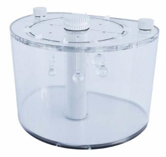
The phantom for evaluating performance of positron emission tomographs (PET). Recommended for use in the evaluation of reconstructed image quality in whole body PET imaging. For simulation of whole-body imaging especially using PET and camera-based coincidence imaging techniques.
