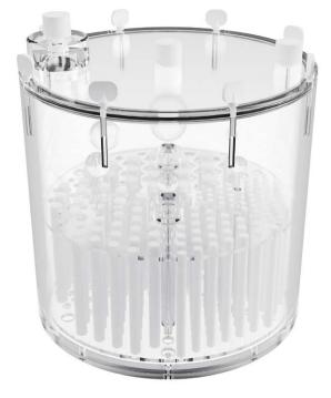
The phantom for NM and PET systems performance evaluation (collimator, artifacts, calibration, reconstruction parameters). It can be used to evaluate, for example: center-of-rotation error, non-uniformity artifacts, changes of radius-of-rotation on spatial resolution, reconstruction filters on spatial resolution, attenuation and scatter compensation.
