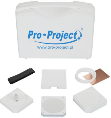
The Pro-Dent set is a universal set of phantoms for carrying out constancy and acceptance tests of conventional and digital dental X-ray units (intra-oral, panoramic and cephalometric).
