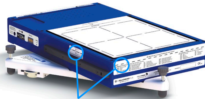
Alignment marks facilitate the TomoTherapy® laser accuracy test (D6)
